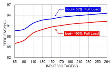
Efficiency vs. Input Voltage TAF300US24 with Forced air cooling
